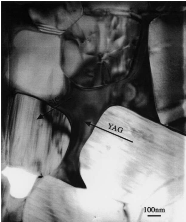
Fig. 8. Bright field TEM micrograph of a YAG crystal located between \alpha -SiC grains.
